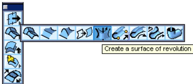
30. Pick the upper line that we just created as the profile to revolve. Then, click both endpoints of the center line.
