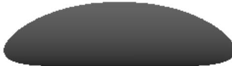
42. Thicken it with the **Solid Thicken** tool. Make sure to hold the CTRL button to thicken it inside.
