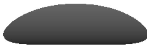
42. Thicken it with the **Solid Thicken** tool. Make sure to hold the CTRL button to thicken it inside.
