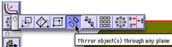
Select the surface you just created, hold down the **CTRL** key on a PC or the **Option** key on a Mac mirror a copy of the surface about the **midpoint** of the gear.
