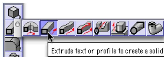
Select the whole gear profile to extrude. Draw a selection fence around the whole drawing as shown below.
