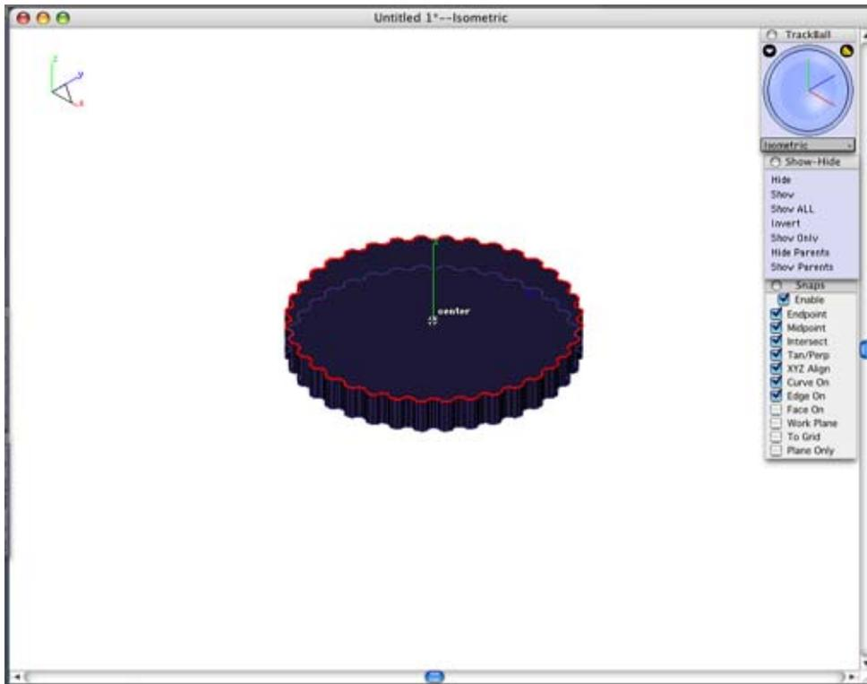
Type in **1.75** inches for the Diameter as shown below and press **Enter**.
