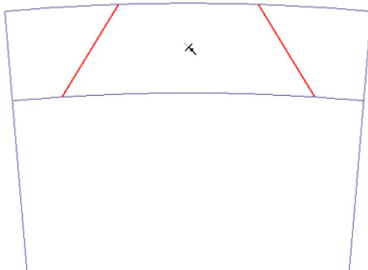
Now we have to select the parts of the arcs to be trimmed away. On the upper arc select the two parts **outside** of the two line. On the inner arc, select the part **inside** the two lines. Your tooth should similar to the one below.
