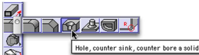
Set the options in the message line as shown below. We are making a **Simple hole** all the way **through** the gear and **normal** to the face of the solid.
