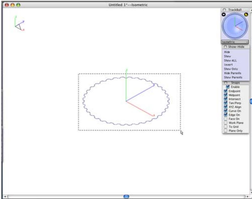
Now it needs a direction to extrude the profile. Select the **origin** for the first point and straight up along the **Z-axis** for the second.
