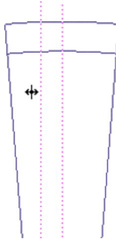
Next, we will do the exact same thing for the right side. You can drag a new line off of the center construction line or you can just enter a negative value in the status line (**-0.10**), and hit the enter key and a new construction line is created.
