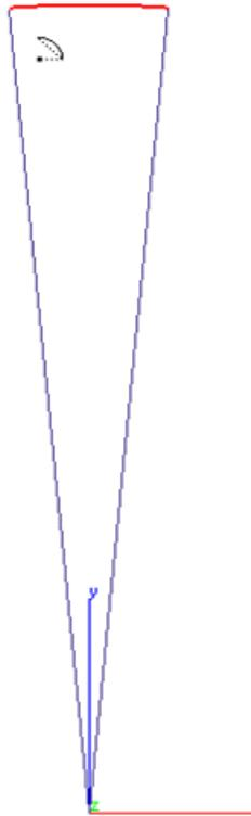
The other two points that it needs are the points along the arc. Select the two endpoints of the lines for those points. The arc created should look like the image below. You can hit **CTRL+F** on Windows or **Command+F** on a Mac to fit the model to the screen (this is the shortcut for Zoom All). You could also go to *View>Zoom All*.
