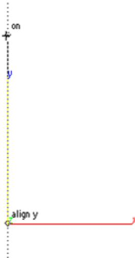
After placing the last point, type **3** into the **L (Length)** field and **95** into the **A (Angle)** field. This will give us exactly the size line we need.
