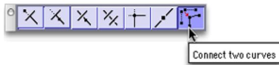
While holding **CTRL** on Windows or **Option** on a Mac select two of the lines that are touching. This joins those two into one piece of geometry. Repeat this to join all four lines.
