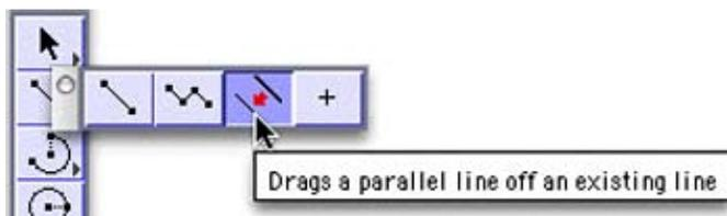
Select the construction line that we created and drag it to the left. After dragging, type **.1** into the Offset field. This sets the offset to exactly **.1** inches.
