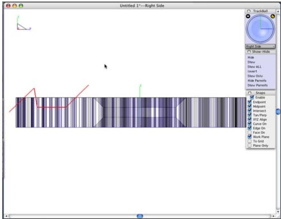
The lines we created are connected at their endpoints, but they are not one piece of geometry. When we create our surface from this piece of geometry, if the pieces are not joined, four separate surfaces will be created (one for each line). The Connect two curves tool has an option to join lines so that we can avoid this situation.
