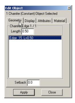
We can change this amount by selecting the edge and changing the value in the *Length* field. Change the number to .125. This will make the chamfer 1/8 inch all the way around.
