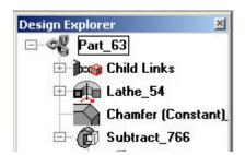
If you remove the Subtract Feature from the list, you will in turn remove the grooves. To do this, right click on Subtract in the Design
