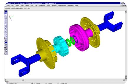
Above: Speakes used Cobalt CAD and 3D modelling software to reverse engineer the Ferrari's missing cam and pawl differential.
