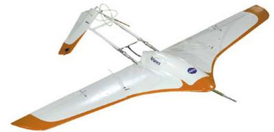
The Kitty Hawk III, created in Graphite CAD software, was the first Mars Flyer design to be tested and built. It set an altitude record for unpowered flight. A new, powered version is now in design using Cobalt CAD and 3D modeling.
