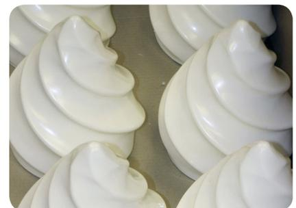
Cobalt's 3D surface modeling (middle) enabled six swirl designs to be prototyped using STL (above) for evaluation.
