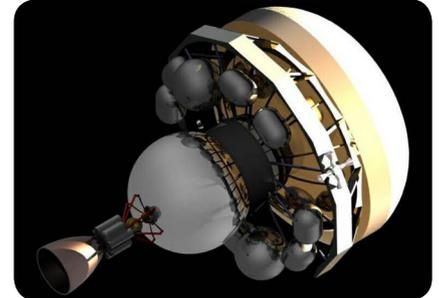
Jones designed the truss structure for the Instrument Deployment and Return Vehicle (IDRV) starting with a rough concept in Graphite precision drafting software, then brought that file into Cobalt modelling software to create and render a full 3D model.
