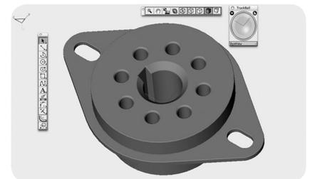
This Cobalt screen capture from THD Electronics, shows a 3D model of a phenolic octal relay socket that is essentially a copy of the old Amphenol tube socket from the '50s.
