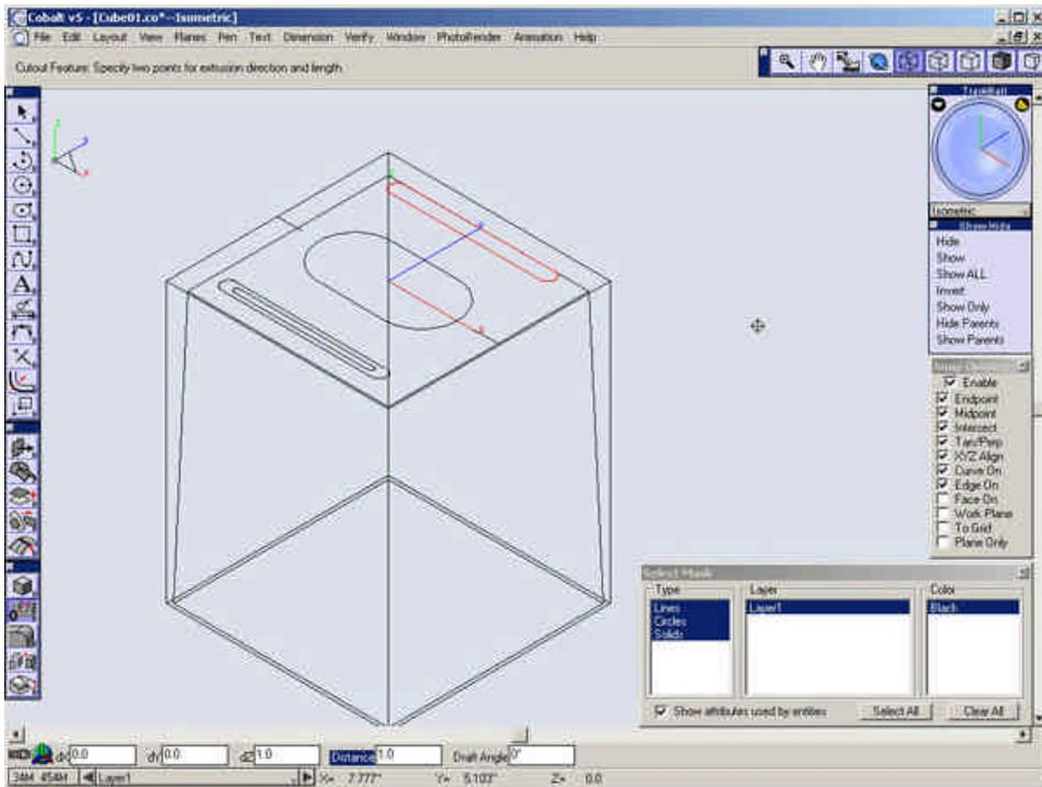
Make sure the **Work Plane Snap** is unchecked. Select one point in space then a second point down in the Z-direction to define the direction of the cutout.
