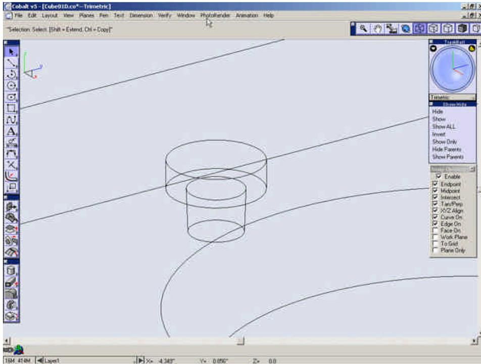
Select the **Cylinder Primitive** tool. Enter **3/8"** for the **D** field (Diameter).
