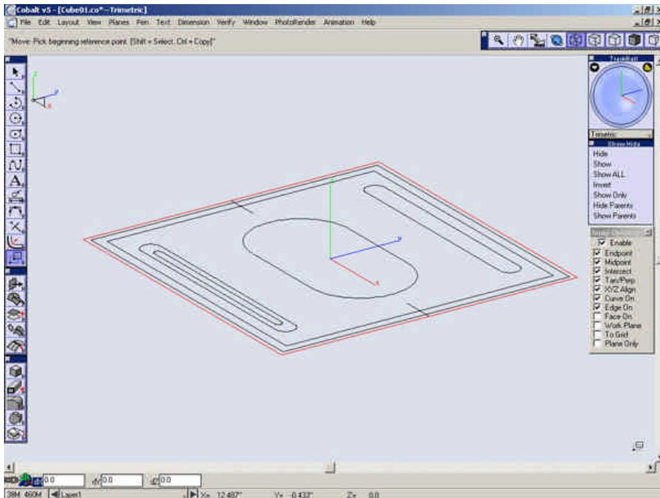
While holding **CTRL** (**Option** on Macintosh) move a copy of the square down along the Z-axis.
