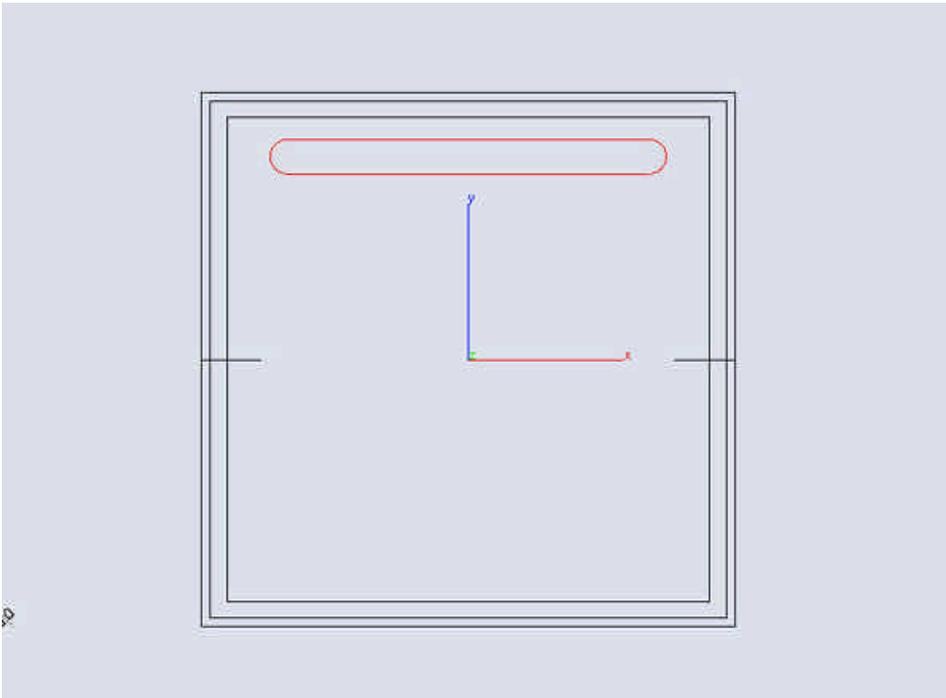
While holding **CTRL (Option)** on a Macintosh, click in the origin and then at a point to the left or right along the X-axis.
