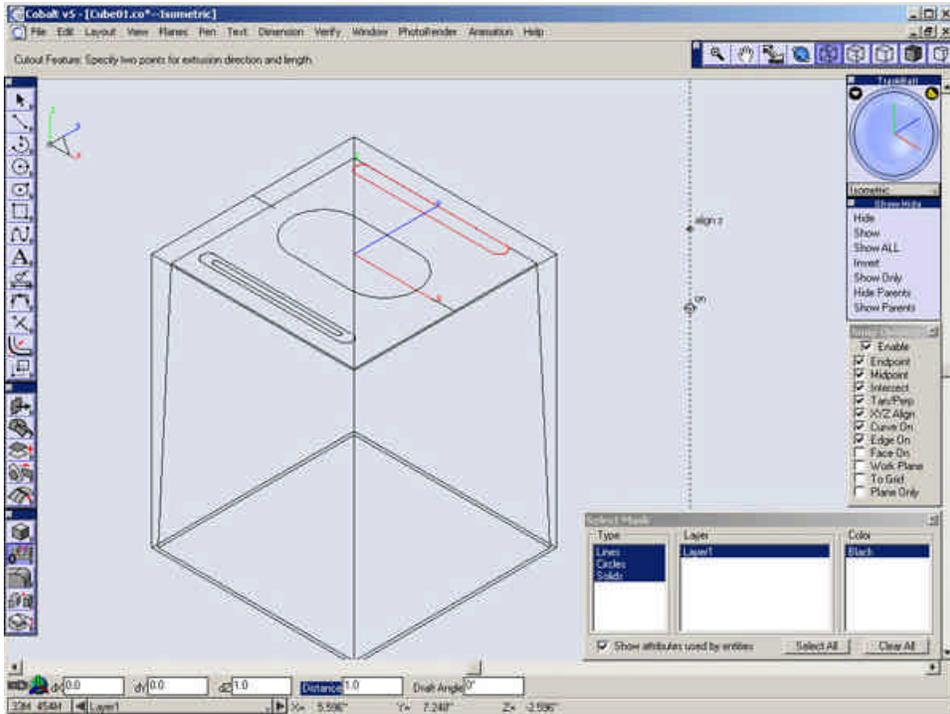
Repeat this procedure with the same solid outer case and the oval shape in the middle of the model. This time, after you define the direction of the cutout, change the value in the **Draft Angle** field to **-30**.
