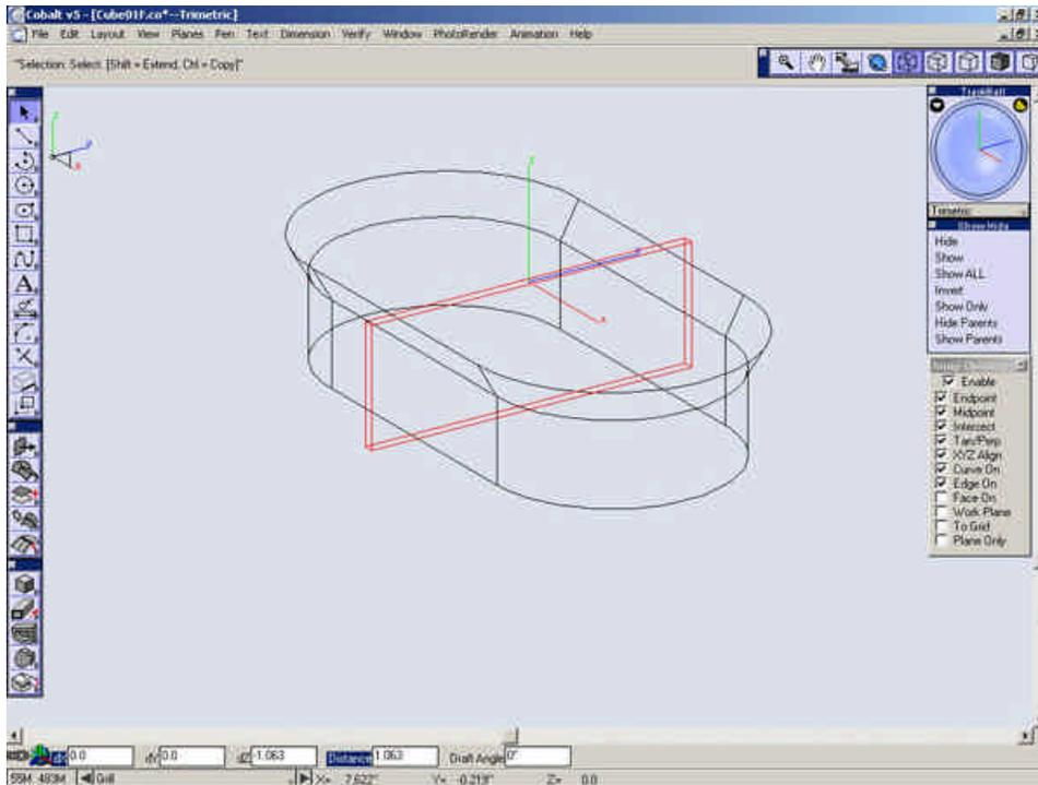
Go to the **Top** view and turn of the **Work Plane** snap.
