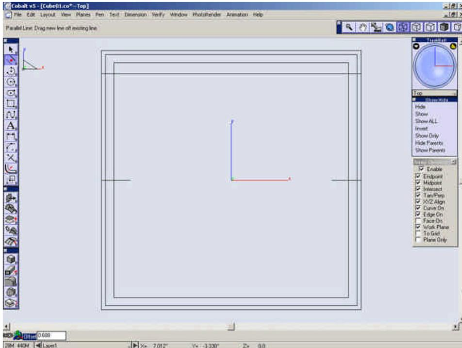
Type **11/16"** into the offset field and press **Enter**.
