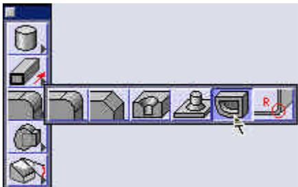
Set the Offset value to **1/16"** and select the Extrusion.
