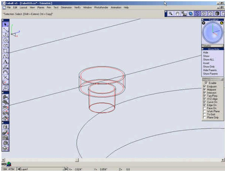
Go to the **Top View** and **Zoom All** and turn the **Work Plane** snap on
