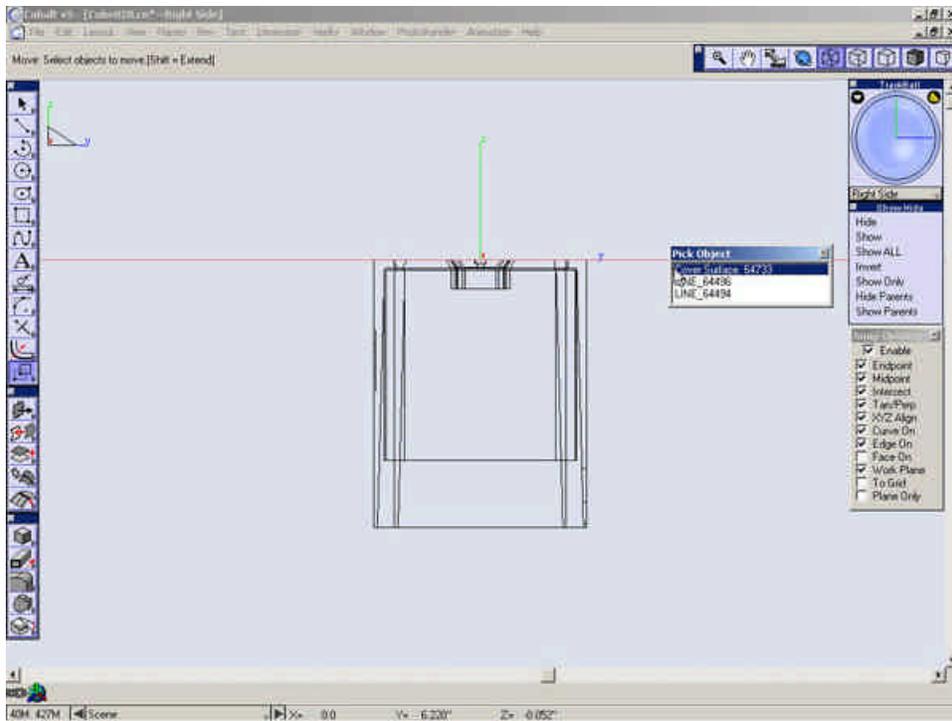
Move the surface to the bottom of the outer case.
