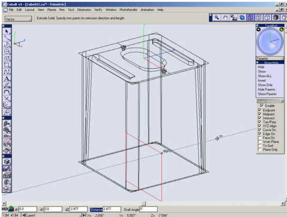
Select the **Radial Blend** tool and set the **Radius** to **1.25**”.
