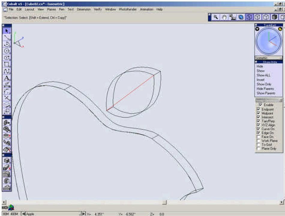
Create another line for the midpoint of the new line out along the Y-axis **1/16"**.
