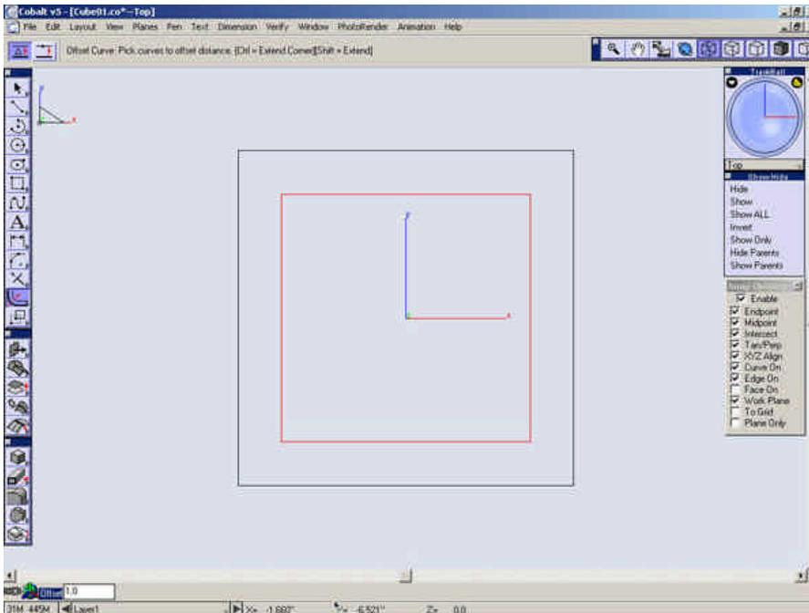
Type **.125**” into the offset field and press **Enter**.
