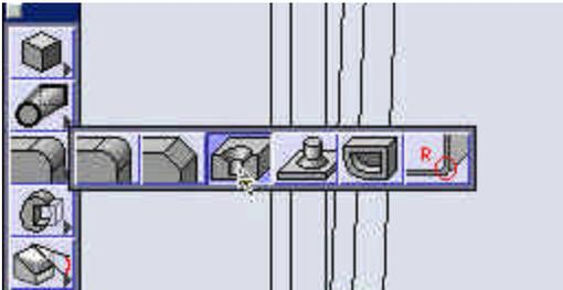
Select the **Counter bore** option and **Through** for the depth.
