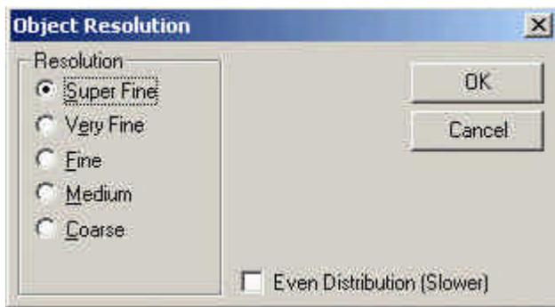
This will only change the resolution of the selected geometry. In order to change the resolution for all geometry that will be created, it is necessary to change the settings in the preferences.
