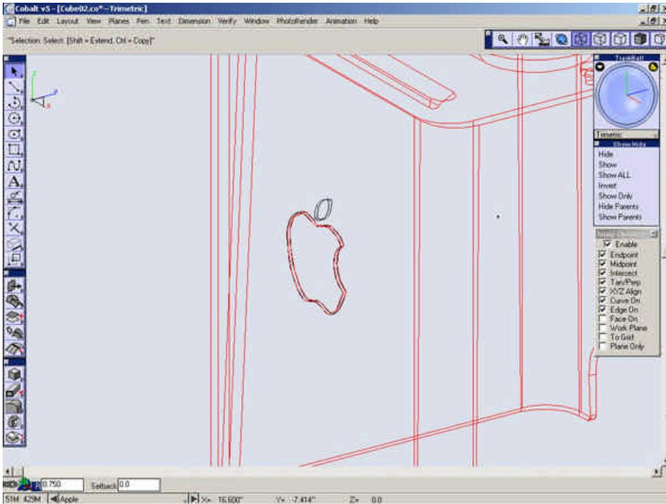
Repeat the extrude and subtract procedure for the smaller portion of the apple geometry.
