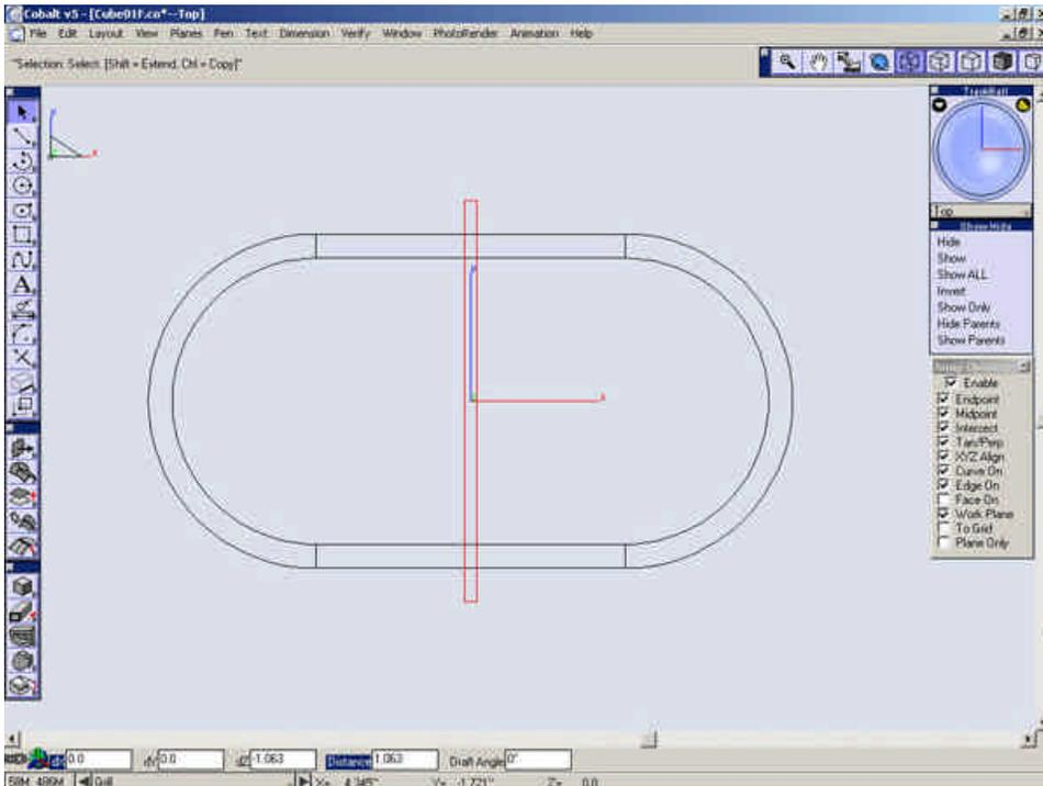
Go to the **Trimetric** view and turn the **Work Plane** snap off.
